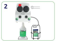
Use the Eco-Multi machine to dilute correct amount of product into a 750ml trigger spray.
